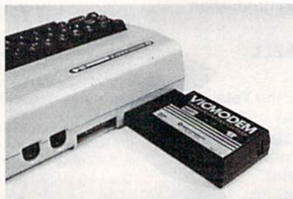
The VICmodem plugs into the user port of a VIC-20 or Commodore 64. A modular cord then connects it to the telephone.
